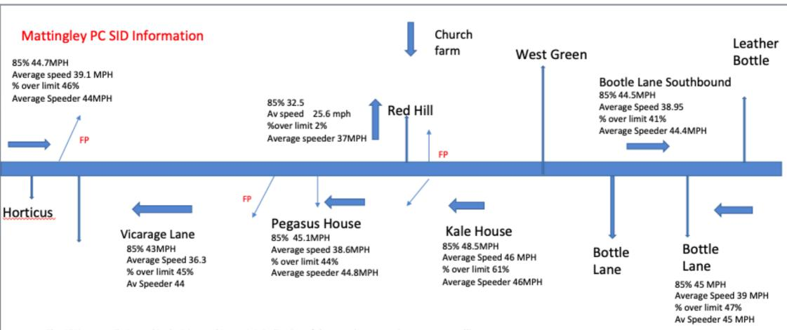
The 85% percentile is used in decision making as it is indicative of the speed most road users are travelling at The theory is that
